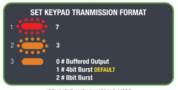
APPLICABLE WHEN IN WIEGAND MODE PRESS \*\* TO EXIT PROGRAMMING
